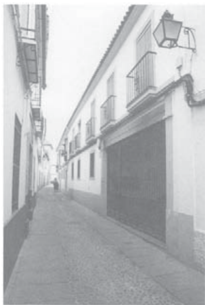
Fig. 4. Calle La Palma. Córdoba, Spain. The narrower the street, the wider must be the garage door to accommodate the turning radius of even a small automobile.
